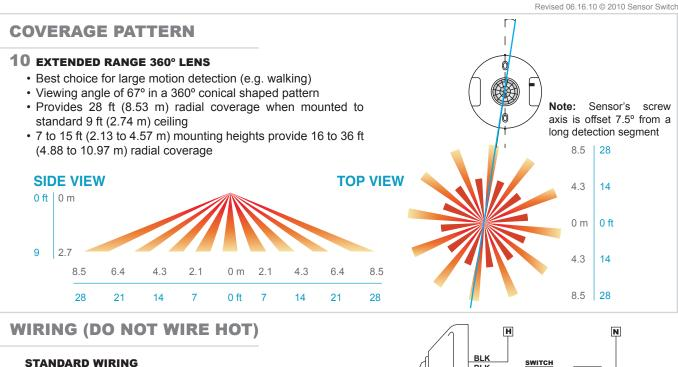
BLACK\* - Line Input BLACK\* - Load Output \*BLACK wires can be reversed WHITE - Neutral
